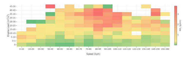
Speed vs Engine Load vs NO<sub>x</sub> (g/km)
